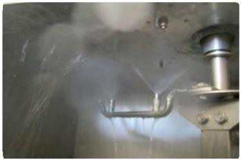
6. Optional Turboclean air fogger cleaning system to blow out and thoroughly clean the connections and feed valve discharges after each feed distribution.
